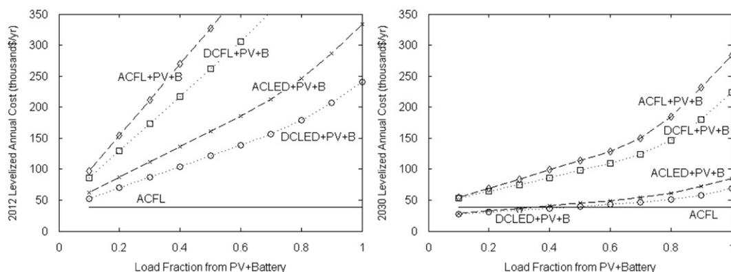
**Fig. 7.** 2012 and 2030 lighting system LAC projections vs. fraction of load provided by solar PV and batteries
