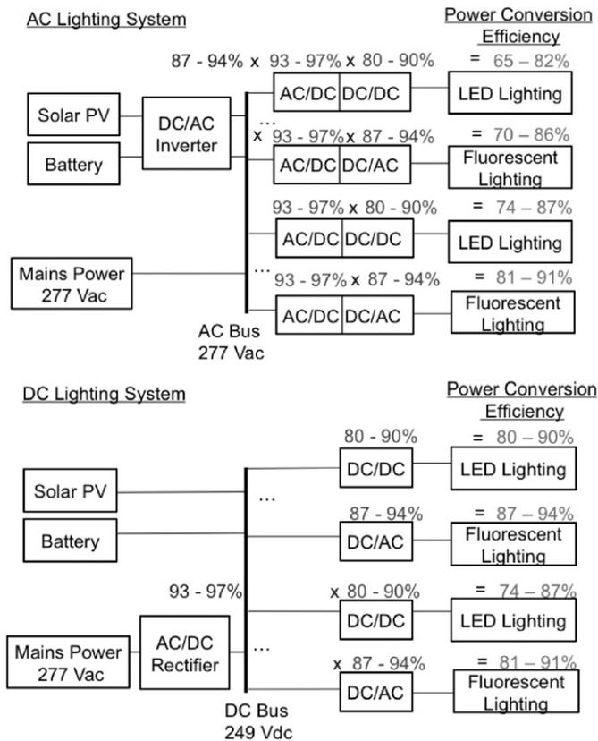
Fig. 1. Schematic of commercial office building lighting system with AC vs. DC architectures. If lighting fixture-level DC/DC power supplies could be eliminated for LED lighting systems, power conversion efficiencies would be improved to 93–97%. DC lighting systems could provide 8–17% greater power conversion efficiencies when used with grid-connected solar PV and battery back-up. Sources: (Jimenez, 2005; George, 2006; Pratt et al., 2007).
