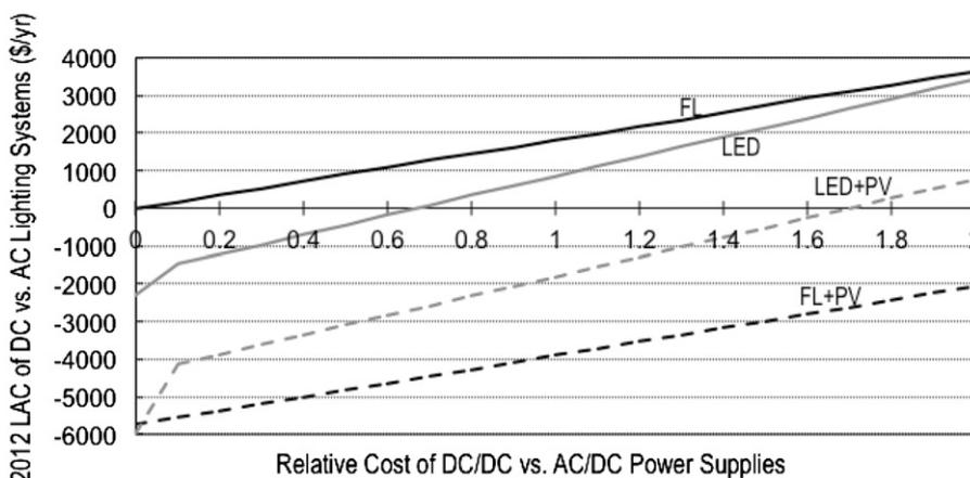
**Fig. 5.** Economics of DC lighting systems depend on the relative cost of DC vs. AC load power supplies, i.e. fluorescent lamp ballasts and LED drivers. Each scenario compares the LAC of the DC lighting system minus the LAC of the AC lighting system.
