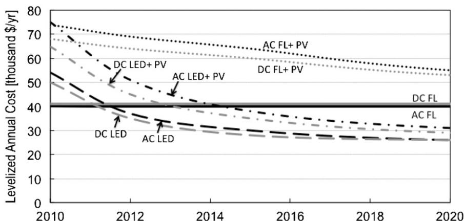
**Fig. 4.** 2010–2020 LAC projections for grid-connected AC vs. DC fluorescent and LED lighting systems. Results do not decline significantly between 2020–2030 and are excluded from the figure. The electricity price assumed is \$0.10/kWh, and the discount rate is 12%. LED projections are from DOE R&D targets (2011b) and solar PV projections are from Curtright et al. (2008). These results assume that DC circuits eliminate the need for LED drivers and a PV inverter.
